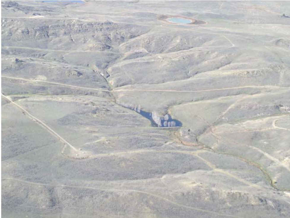
Figure 2. CBM development landscape in the Powder River Basin of Wyoming. Note the roads, pods of well heads, and in-channel and off-channel product water impoundments. http://waterquality.montana.edu/docs/photo/cbm_landscape.shtml
