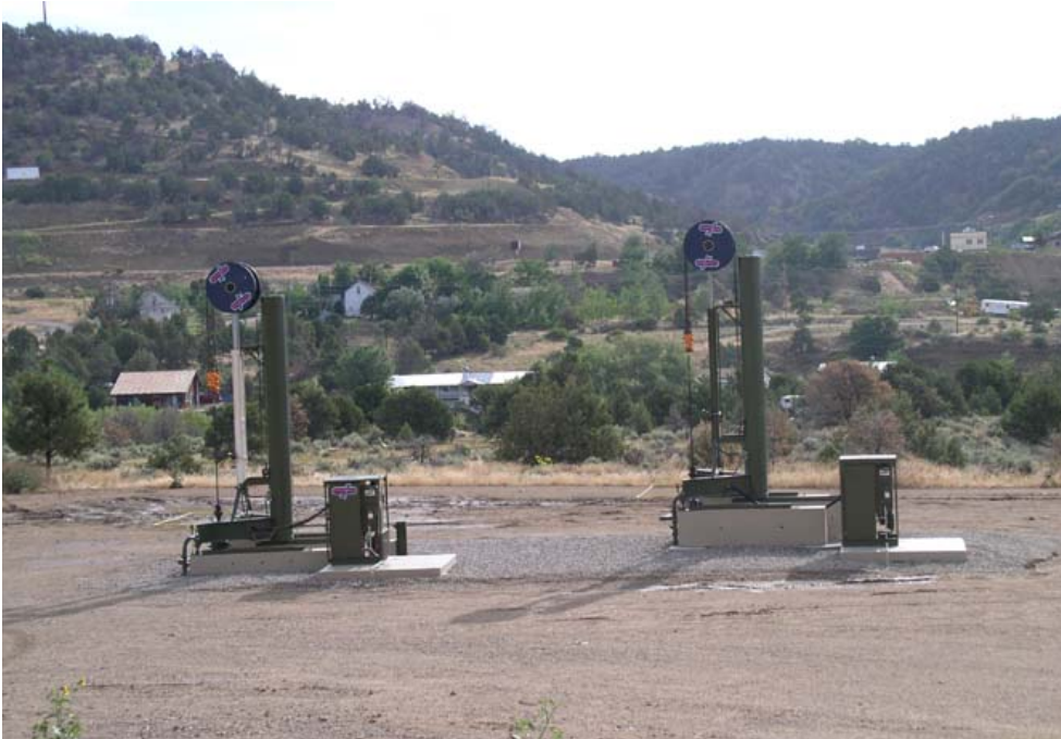
Figure 9. Progressive cavity pumps located very near the city of Durango, Colorado, in the San Juan Basin. These pumps are a best engineering practice to reduce noise typically associated with CBM wells.
