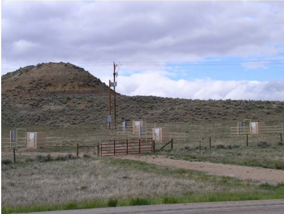
Figure 4. Pod of well heads in the Powder River Basin of Wyoming. Each well is drilled into a different CBM-producing coal seam.
